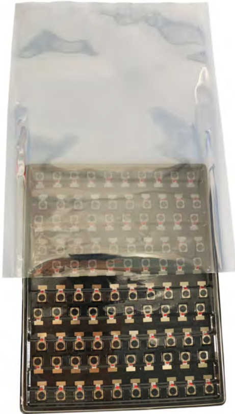
Place Tray into Anti-Static Bag
