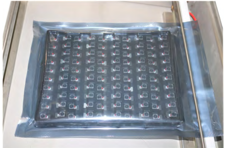
Vacuum the Anti-Static Bag
